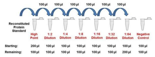
6. For samples of unknown protein concentrations, serial dilute the experimental sample using Sample Diluent B to determine range of
