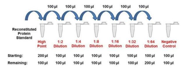
For samples of unknown protein concentrations, serial dilute the experimental sample using Standard & Sample Diluent to determine range of detection and acceptable dilutions. Shown below is a diagram illustrating a 10-fold serial dilution on a given Sample of Interest.
