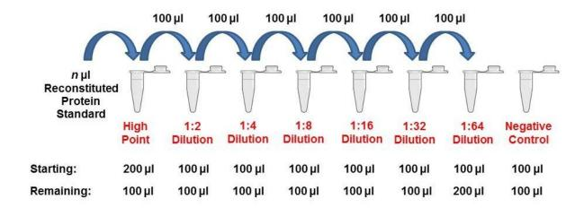
For samples of unknown protein concentrations, serial dilute the experimental sample using Assay Diluent to determine range of detection and acceptable dilutions. Shown below is a diagram illustrating a 10-fold serial dilution on a given Sample of Interest.
