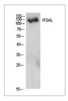
Western Blot analysis of 293 cells using Integrin  $\alpha L$  Polyclonal Antibody. Secondary antibody(catalog#:RS0002) was diluted at 1:20000
