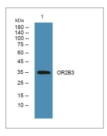
Western blot analysis of lysates from K562 cells, primary antibody was diluted at 1:1000, 4°over night
