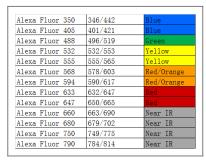
To use the Alexa Fluors with fluorescent imagers, use a spectral line of the blue laser diode for Alexa Fluors 405, a cyan (488 nm) laser for Alexa Fluors 488, a yellow (526 nm) laser for Alexa Fluor 550 or 594, and a red (633 nm) laser for Alexa Fluor 649. The Alexa Fluor 680 and 790 fluors are compatible with laser- and filter-based infrared imaging instruments that emit in the 700 nm, and 800 nm
