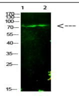
Western Blot analysis of 1,mouse-liver 2,hela cells using primary antibody diluted at 1:1000(4°C overnight). Secondary antibody:Goat Anti-rabbit IgG IRDye 800( diluted at 1:5000, 25°C, 1 hour)
