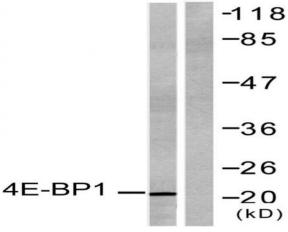
Western blot analysis of lysates from MDA-MB-435 cells, treated with EGF 200ng/ml 30', using 4E-BP1 Antibody. The lane on the right is blocked with the synthesized peptide.
